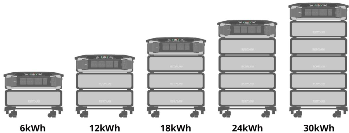
The rated capacity of one battery is 6kWh. To expand capacity for powering your appliances (see **Overview** or **Power Your Appliances**) or backing up your whole home (see Backup System), one can connect up to 5 batteries to an inverter or up to 15 batteries to 3 sets of inverters, which makes the total capacity add up to about 30kWh to 90kWh.
